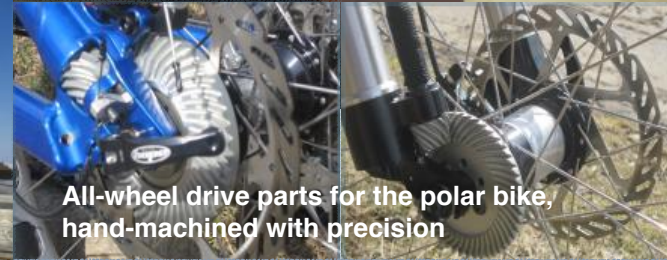
All-wheel drive technology engineered by Christini Technologies, Philadelphia, USA
